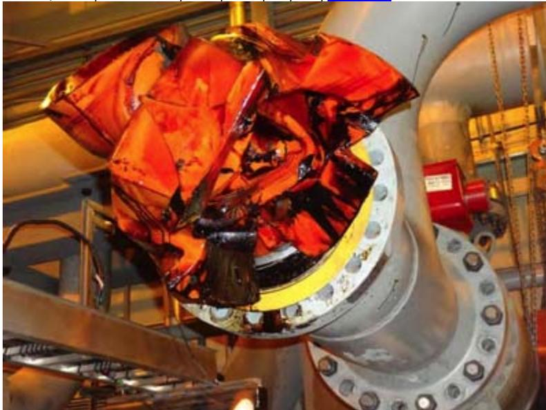
*The damaged scraper pig stuck in relief piping at Pump Station No. 5 in 2010*
