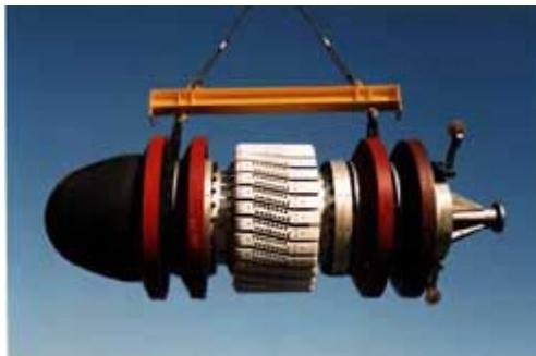
New technologies have made smart pigs even more efficient and effective. Pigs that use magnetic flux leakage (MFL) technology, ultrasonic measurements, and geometric tools are among the most common smart pigs used today.
